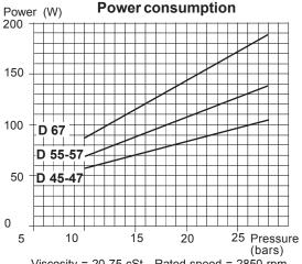
Viscosity = 20-75 cSt - Rated speed = 2850 rpm
